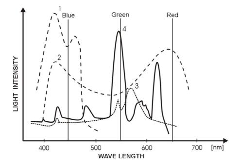
**Fig.1**. Light wave length necessary for plant's: 1 - phototropism and 2 – photosynthesis; Spectral characteristics of the fluorescent lamps used in 3 - SVET SG (LB 6-8) and 4 – SVET-2 SG (DS 11/21) and of the new blue, green and red LEDs.
